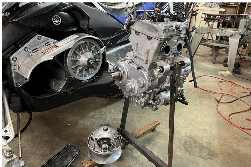
Yamaha Phazer engine after removal from snowmobile ...first glance it could be mistaken for a Rotax 582.
