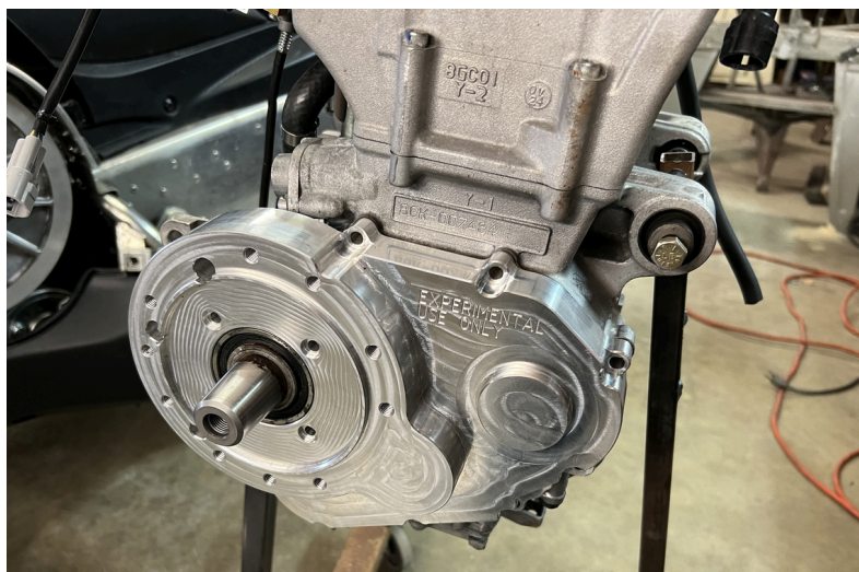
Photo shows adapter plate which replaces the Yamaha gear cover. The Standard Rotax "C" gearbox then bolts directly to the Adaptor.
