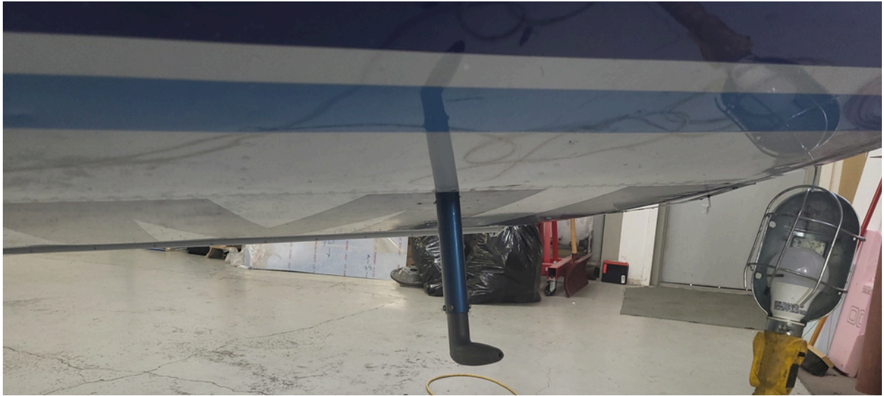
Pitot mast installed on the wing
