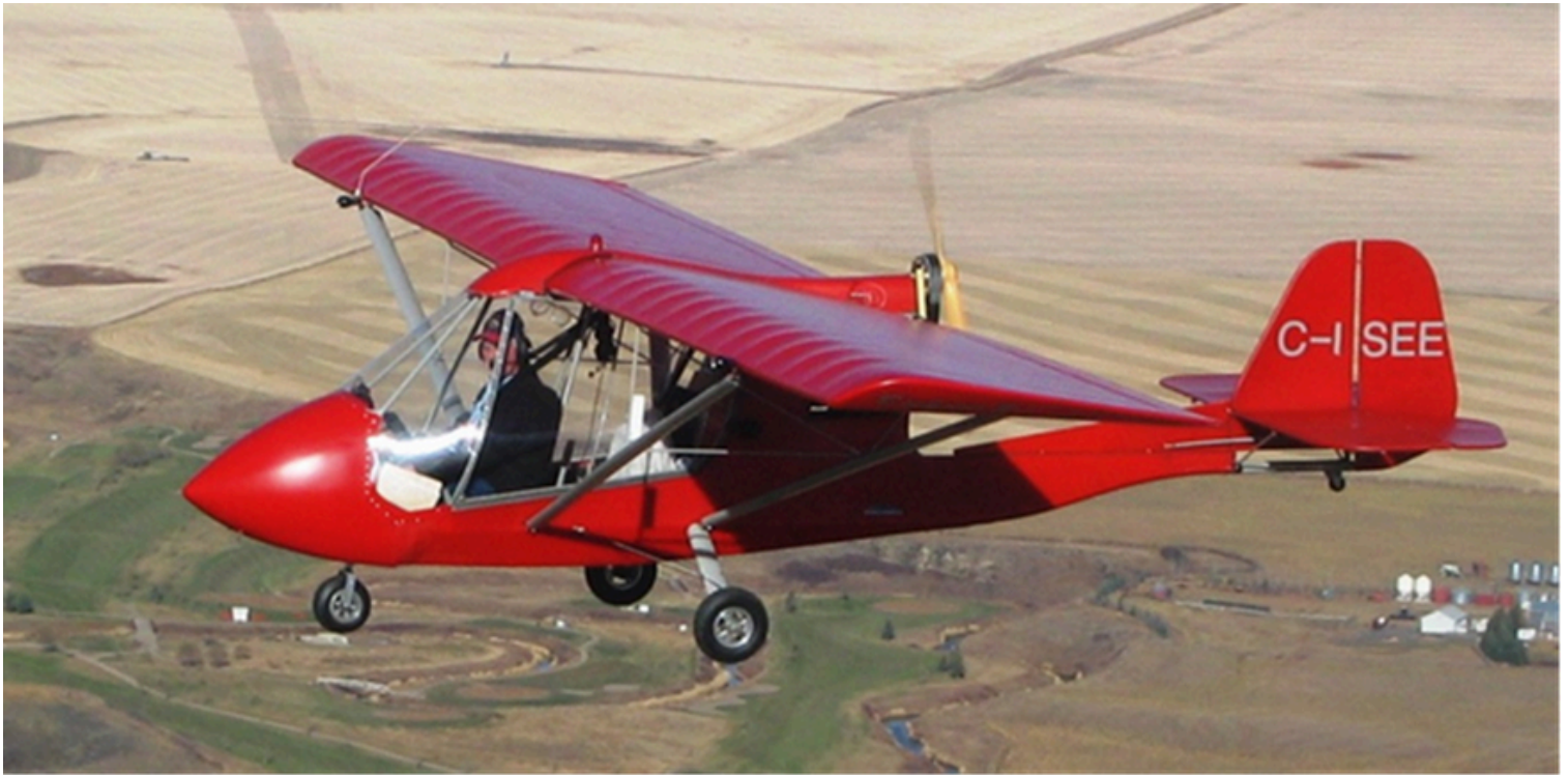
A Quad City Challenger II, built with aluminum tubing typically found in ultralights dating from the 80s, and powered by a Rotax two-stroke motor.
