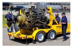
I know many of you probably monitor your engine Cylinder Head Temps, from 2-6 cylinders. How do you monitor them on a 14 cylinder engine during a ground test run? These CHT's were taken manually, while running the engine, with a handheld infrared heat gun, by a crewmember, that's how!
