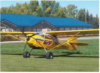
I was able to find a used 912 UL, and combined with an electric IVO propeller I have an ultralight that is a 100mph airplane.
