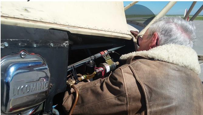
Bob repairs the fuel pump on the ramp at Garden City, KS. By Stu Simpson
