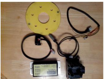
Leburg crank triggered electronic ignition for four cylinder engines. Will work on any four cylinder engine. Comes with Ford Visteon coil, trigger wheel, electronics and manual. Dwell curve built into the electronics. Easy installation. \$ 700.00 invested. Asking \$300.00. Tim Vader, 403 620-3848, vadert@shaw.ca
