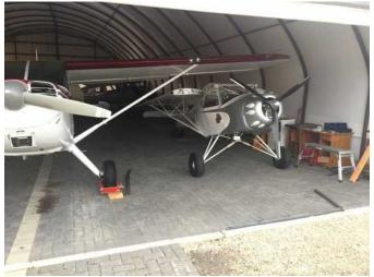
The folding wings of the Kitfox were a necessity because of the available hangar space in Carstairs.
