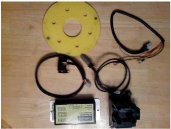
Leburg crank triggered electronic ignition for four cylinder engines. Will work on any four cylinder engine. Comes with Ford Visteon coil, trigger wheel, electronics and manual. Dwell curve built into the electronics. Easy installation. \$ 700.00 invested. Asking \$300.00. Tim Vader, 403 620-3848,
