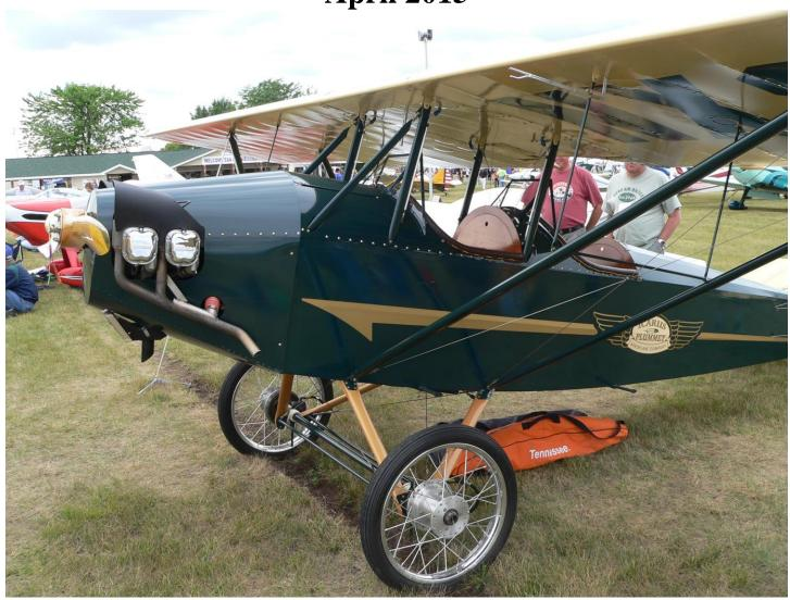
To me, the Pietenpol has always been the Ultimate Ultralight. It's a simple to build plane from plans, all wood for the amateur builder, powered by a multitude of simple and inexpensive engines, has a beautiful, classic look and has good flight manners!
