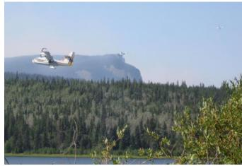
123AF turboprop engines at 2380 shp and Hamilton Standard constant speed 4 blade props. They cruise at 180 Kts. They use 840 liters of fuel per hour and you thought yours swallowed a lot!
