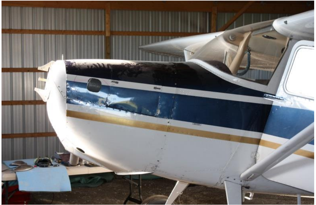
First trial fit of the modified cowl. Blisters yet to be installed.
