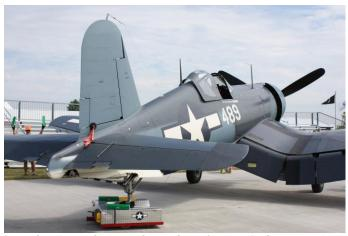
I noticed an interesting aircraft tug being used at Oshkosh. It's made by Trace Towbots and is RADIO CONTROLLED! Essentially, the tug is driven up under the third wheel (tailwheel or nosewheel) and captures it. The airplane can be maneuvered by a radio controller much like you'd see on an R/C car. The real advantage is that you can maneuver the airplane with one person and no need for wing walkers. Obviously, it's powerful as it easily pulled around this Corsair!
