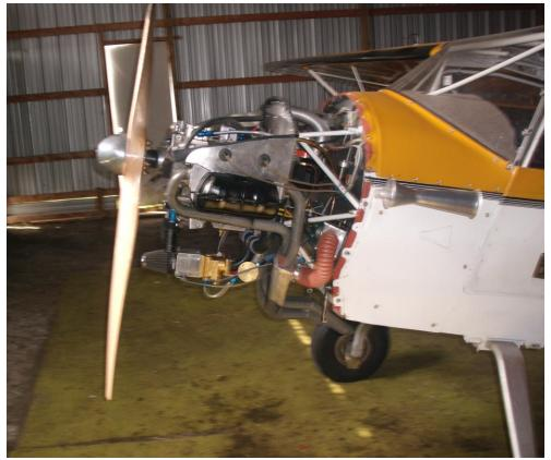
After another 18 months of repairing and changing out carburetors to find one that I felt happy with I settled on my fourth choice, the Rotec throttle body injector. I had tried a Zenith carb and the Aerocarb. I almost didn't settle on the Rotec because the first one sent from Australia had a fuel leak internally and no amount of adjusting would stop it from running rich.
