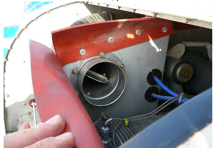
The oil cooler controller can be seen in the upper photo behind the baffles. The photos below show it in the open (top) and closed (bottom) positions.
