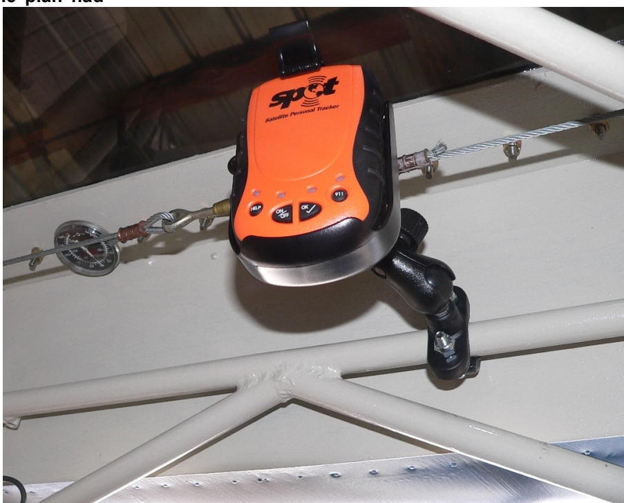
The new SPOT mounting kit uses RAM components to secure your SPOT device.
