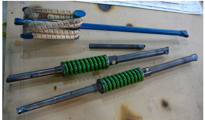
This shows the gear leg ends in various stages of completion. Note the draggy bungee gear above.
