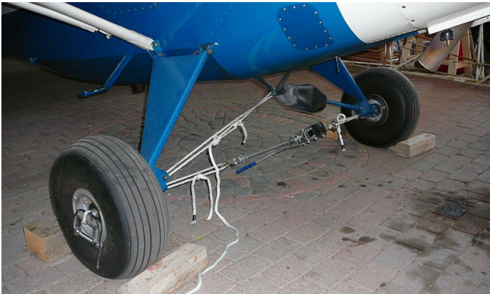
One gear leg removed. The upper rope was installed as a safety rope in case the lower one failed.
