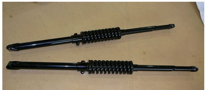
The new gear legs ready for installation. Don't they look shiney!!! This should net at least another 25 mph!
