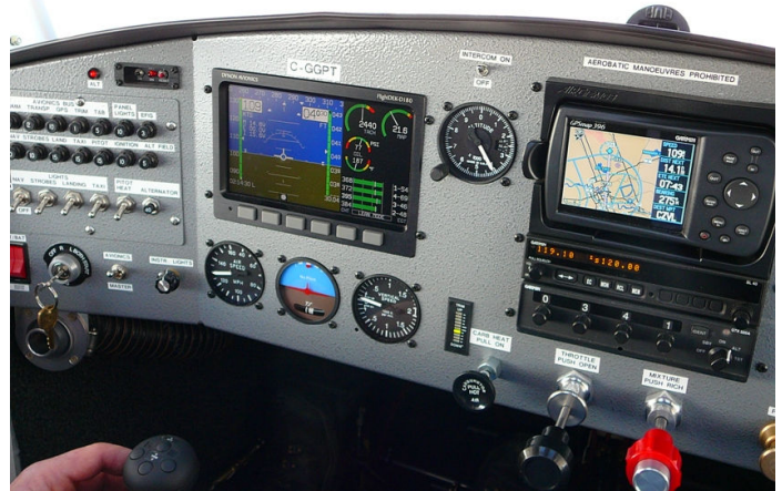
The panel on Gil's Elite shows a well designed layout. The Dynon makes for an elegant solution to a clutter panel.
