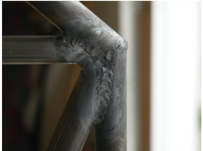
This photo shows two types of joints. The two tubes on the right were joined with a butt weld from a bevel cut. The other two tubes have fish mouths cut in the ends.
