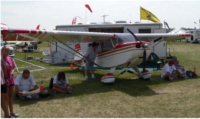
The venerable, all-wood Dakota Hawk provides some well needed shade. This aircraft is now available as a plans-built plane.
