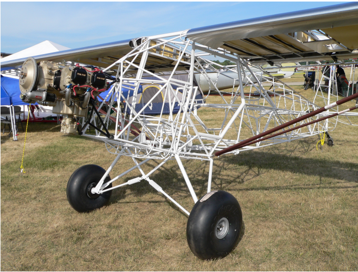
Another "renewed" design. This PA-12 super Cruiser kit comes complete as pictured (less engine) from Smith Aircraft. They also sell a PA-18 Super Cub kit.
