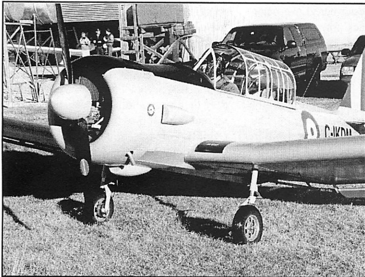
Dan Mitchell's EZ-Harvard with new Oleo strut landing gear designed and built by Dan and Ted Beck. Photo by Adam Hunt.
