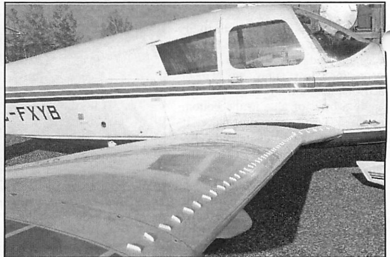
The vortex generators installed on the right wing.
