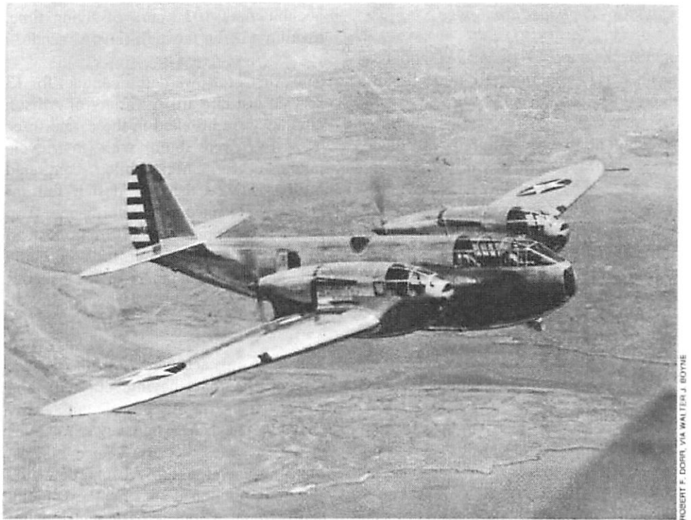
Designed by young engineer Robert J. Woods, the radically different Airacuda incorporated twin pusher engines driving three-blade propellers via an extension shaft.
