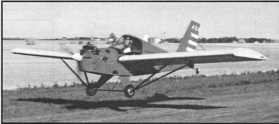
Carl takes off with his 3-blade Ivo prop as part of his propeller testing program.
