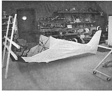
Photo 1 - fuselage envelope installed
