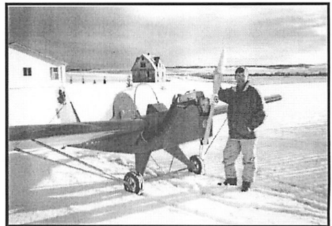
Dale Robinson and his miniMAX on Dave Bolton's strip. He's using a Rotax 447 for power. He designed his own canopy.
