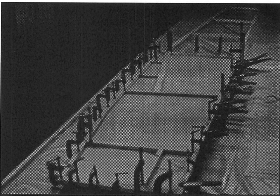
A Sea of C-clamps hold plywood to the left-side fuselage frame.
