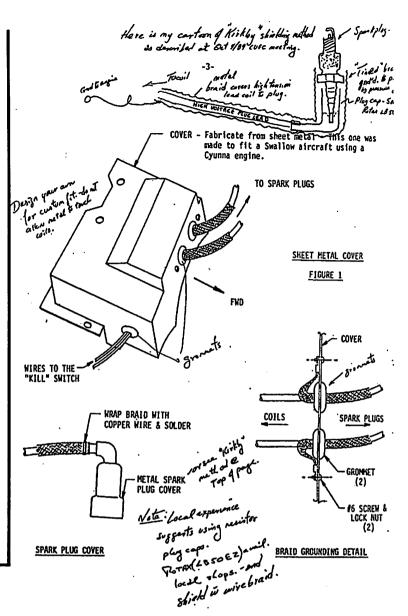
AN communication equipment installed in an ultralight aircraft will operate satisfactorily if properly installed and protected from the high energy ignition system.
